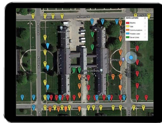
A screen capture from the asset location map in the InfraMarker app, used for the installation of RFID Markers in 2015.
